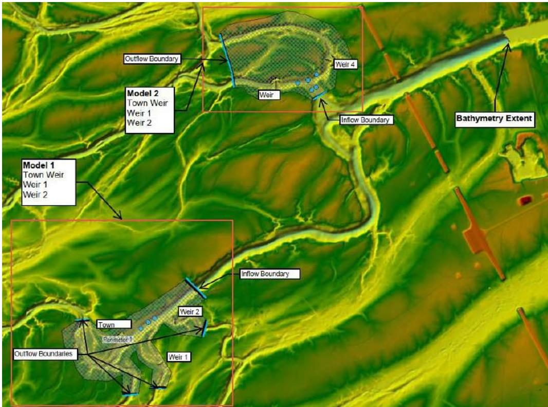
Figure 7.1:HEC-RAS Model Set Up
